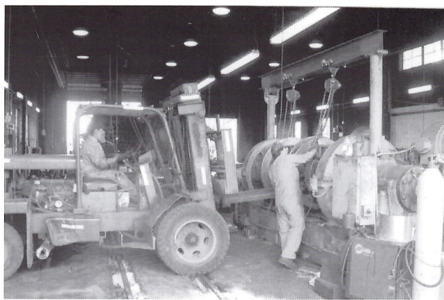
Tommy Garcia brings a set of drivers to the wheel lathe in the Chama shop, while Steve Montano guides the drivers into place.
