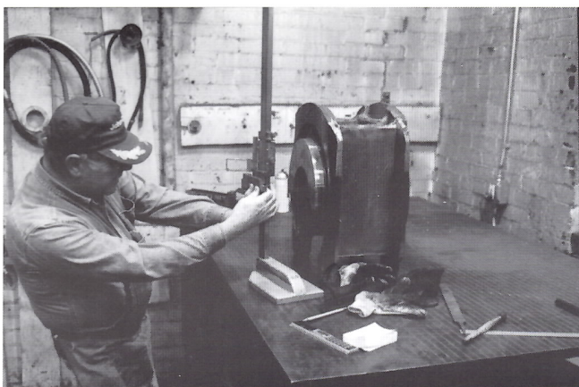
Bob Triggs setting up to measure faces on a driver box for 484. Below, two sets of drivers with new tires under 484. (Photos by Tom Cardin on February 3, 2004, except where noted.)
