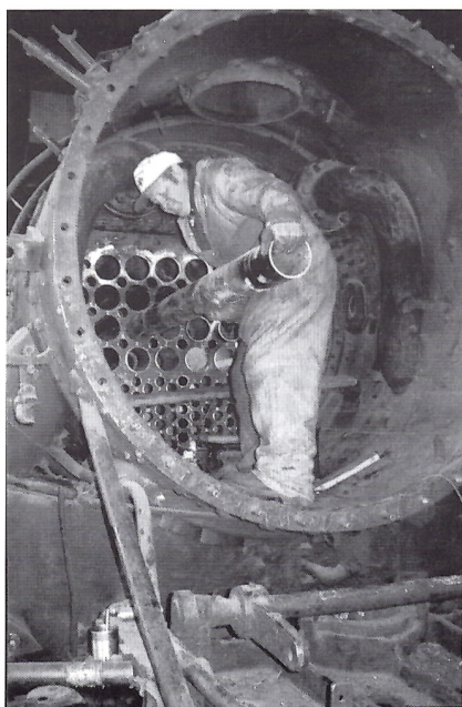
In Chama Rickey Rivas finishes loading a superheater flue in engine 484 (January 28, 2004).
