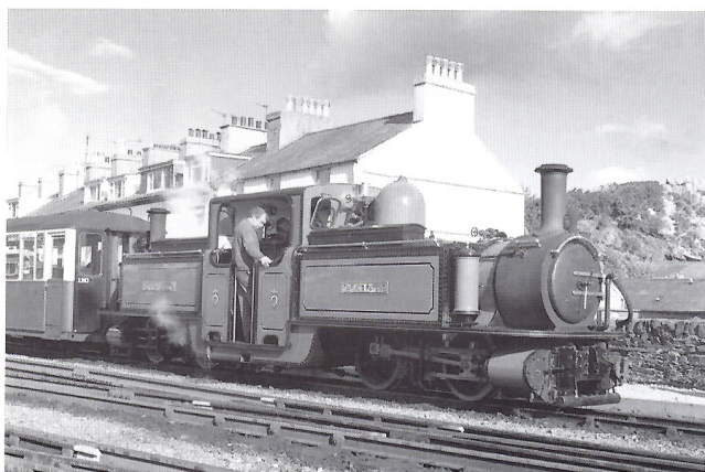
David Lloyd George at Porthmadog: Built at Boston Lodge in the early 1990s to traditional FR outline and style, double Fairlie David Lloyd George is the most powerful locomotive on the FR thanks to increased boiler pressure and superheating. (Photo by John Dobson.)
