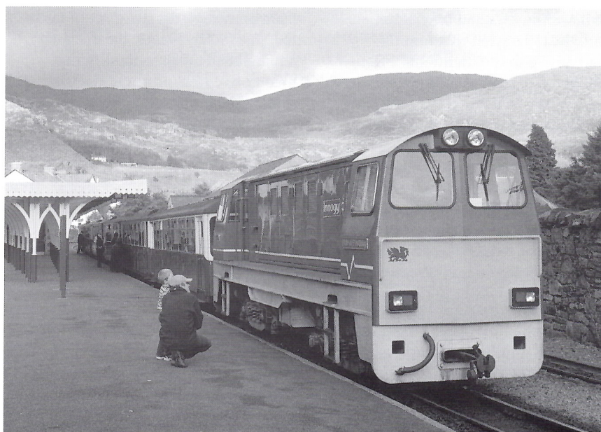
Vale of Ffestiniog at Blaenau Ffestiniog: In the mid 1990s the FR acquired two centre-cab diesel locomotives with almost new 350hp Cummins engines from a South African cement company. One went to the Welsh Highland Railway project more or less as received, the other was considerably modified to reduce its height for use on the FR. The result is a powerful, economical and extremely useful double-cab machine. It acts as standby to the double Fairlies on heavy summer trains and is also used for lightly loaded 'off-peak' trains. (Photo by Peter Treloar.)
