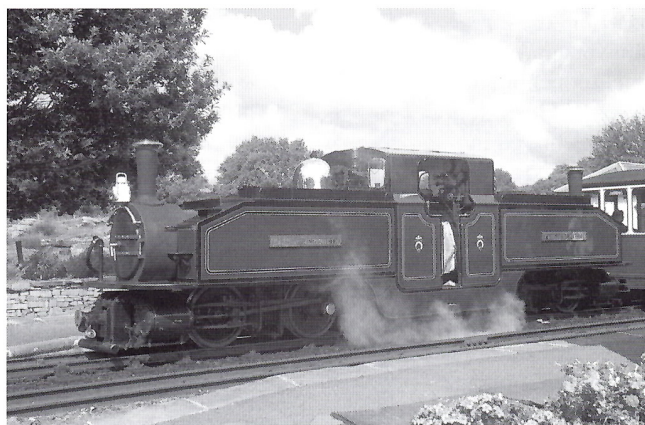
Earl of Merioneth at Minffordd: Double Fairlie Earl of Merioneth was the first new steam locomotive to be built at Boston Lodge during the preservation era, going into service in 1979 – the first locomotive built by the FR since 1886. Its angular styling has earned it the nickname of The Square . (Photo by Peter Johnson.)
