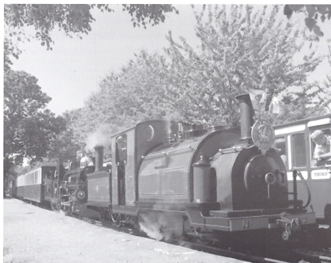
Prince at Minffordd: Double-heading with Linda on 3 August 2003. The headboard and flags are to mark 140 years of steam power on the FR. Compared with Palmerston, Prince has suffered elephantiasis since the 1950s, the smokebox, tanks and cab all having been enlarged to meet modern needs and the frames strengthened. Known affectionately as 'The Old Gent' Prince is now oil-fired and superheated and can haul up to 6 carriages with relative ease. (Photo by Chris Jones.)
