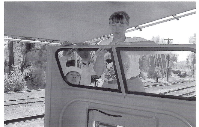
Noreen Breeding (l) and Laura Kammerer install weather strip in a Fairmont speeder's window (session D).
