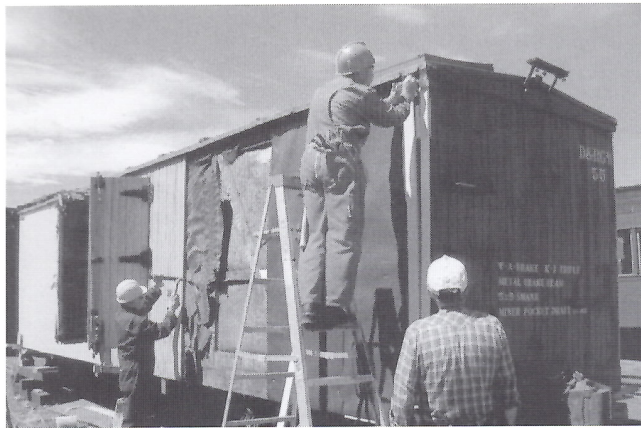
Jay Samuels (l) and Matt Jameson remove sheathing from short refrigerator car 55 in Chama during session E.
