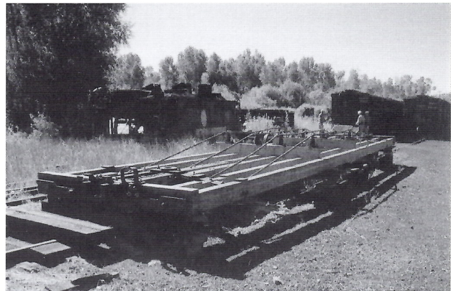
Flat car 6314 being rebuilt in Chama in the field east and below the engine house. Rebuilding the car upside down makes it easier to install heavy metal components (session D).
