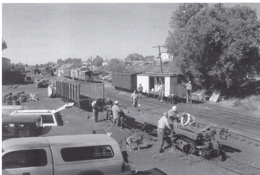
Looking south over the Chama railyard during session D in June. Volunteers are working on pipe gondola 1557 in the foreground. Behind 1557 is high-side gondola 1648. Both cars will be part of a restored pipe train. In the background volunteers are converting concession car 450 back to boxcar 3591. (All photos by Tom Cardin except where noted.)
