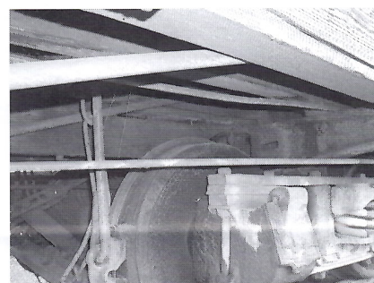
Gondola 1648, center sill separation.
