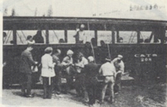
The "draw bridge" steps are lowered for passengers boarding a C&TS train. Plexiglas windows may be raised and lowered depending upon the weather. Photo-Jim Rupley
