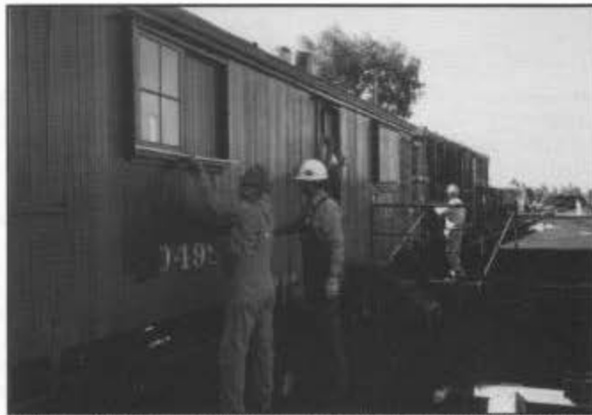
Chama: installing new screening on bunk car no. 04982; work was finished on two of the three bunk cars.
