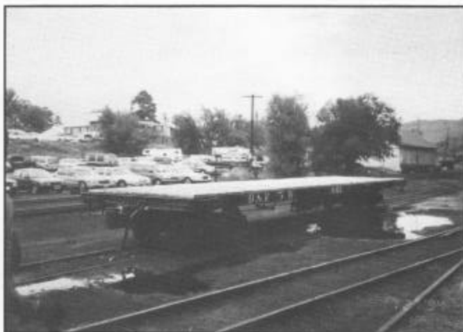
Work on the second steel flat car no. 601 has been completed and linseed oiled at the end of the work session, July 27, 1994. Photograph by Glenden Casteel.
