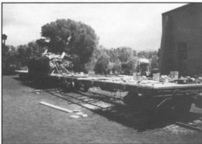
Work proceeding on steel flat car no. 601 with the decking approximately half completed, July 25, 1994.
