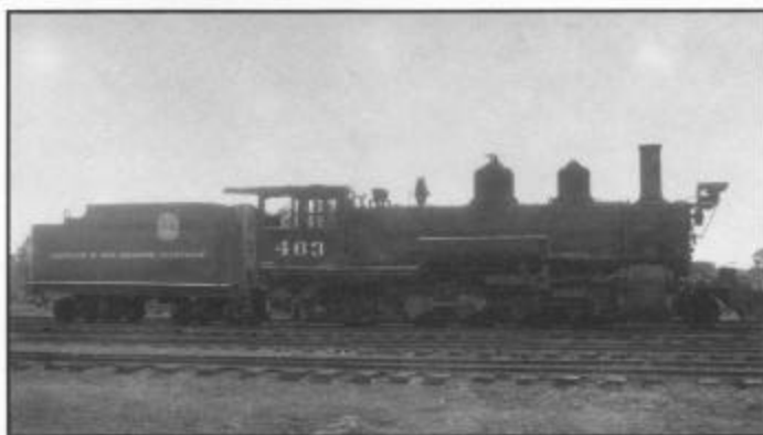
Figure 3. Engine 463 rests in Gunnison, Colorado, on August 31, 1938, after falling through the bridge at Cimarron. The cab roof and the entire left side of the cab is missing. The engine was later hauled to the shop in Salida, where a new cab was built. Robert Graham photo, Tufford Collection.
