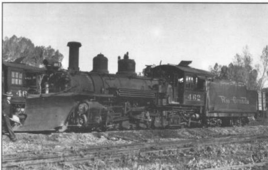
Figure 11. Engine 462 spent many years in the 1940s leased to the Rio Grande Southern, and it is shown here at Ridgway, Colorado, between assignments in May 1947. The engine was the last nonsuperheated K-27 in service, being scrapped in 1950. Part of 462 still exists — the tender was saved as water car W-462, which is in Chama today. Photograph by Gerald M. Best. California State Railroad Museum.
