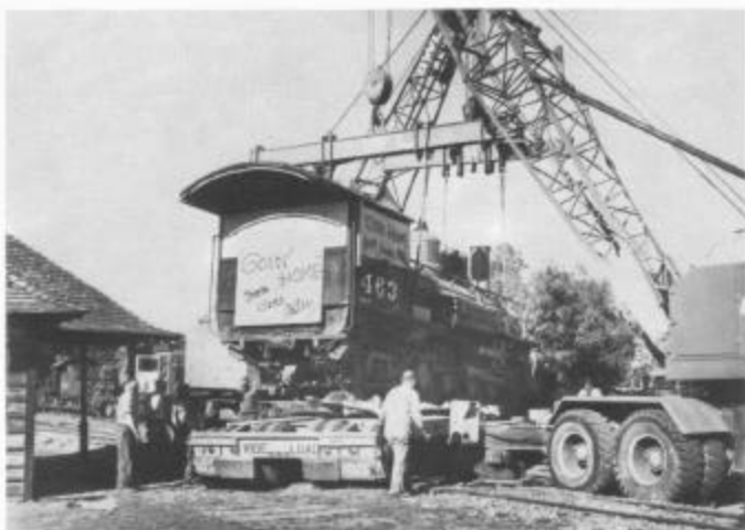
Engine 463 is shown here being lowered on to a second flat bed truck for transport to Saugus. The engine weighed about 66 tons. February 22, 1972. Tom Klinger Collection.
