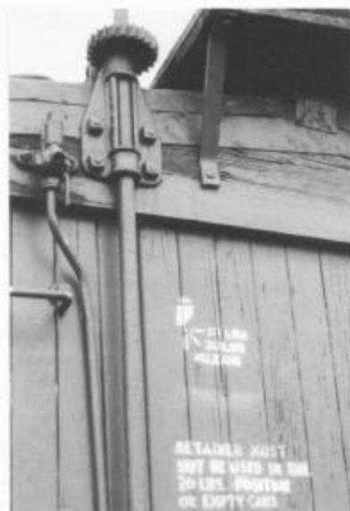
Lettering about the brake system retainer valve is on the end of the car near the brake wheel. Chama, May 11, 1995.
