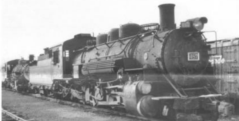
Top: Engine 484 without its plumbing, jacket, and lagging was parked just south of the Chama depot on January 11, 1996. The absence of snow was unusual for the middle of January.
