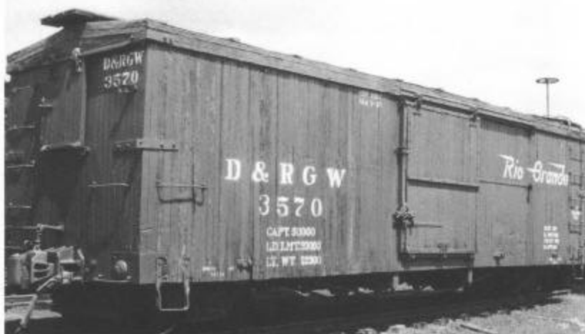
The lettering on a freight car such as boxcar 3570 gives many messages, each one vital to the safe and efficient operation of the railroad. Chama, May 11, 1995.
