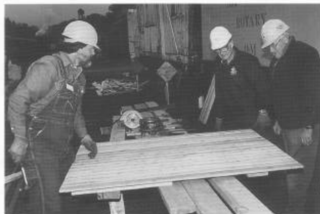
Phil McDonald (left), Warren Smalley, and Roger Briggs make a new coal tender door for rotary OM (session A).
