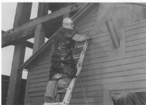
Car 053 after restoration work this summer. Volunteers installed new siding, replaced the clerestory screens and roof walk, replaced the A end platform (shown here being assembled), and painted the entire car. The new siding was fastened with deck screws because it was discovered that one of the side sills was more damaged than originally thought. Its repair will require that the siding be removed at a future work session. Deck screws will facilitate removal; when the siding is reattached, nails will be used.
