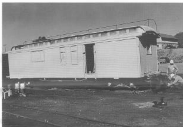
Car 053 after restoration work this summer. Volunteers installed new siding, replaced the clerestory screens and roof walk, replaced the A end platform (shown here being assembled), and painted the entire car. The new siding was fastened with deck screws because it was discovered that one of the side sills was more damaged than originally thought. Its repair will require that the siding be removed at a future work session. Deck screws will facilitate removal; when the siding is reattached, nails will be used.
