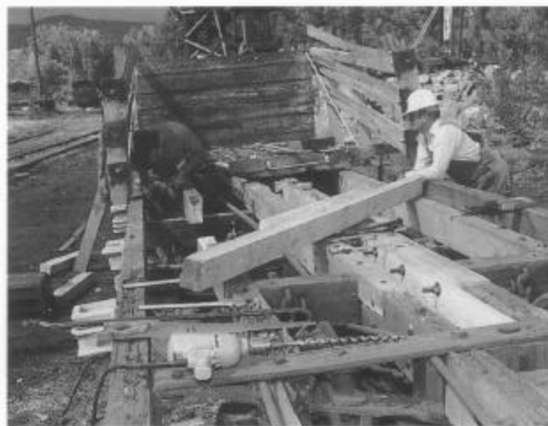
Roy Blizzard (left) and Ken Earle install new intermediate sill pieces on wheel and tie car 06092 during August 1998 mini work session.
