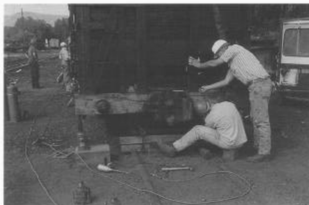
During the August mini work session, Kevin Gilbert (left) and Geof Gordon tighten bolts on the new end sill for stock car 5633. ➔
