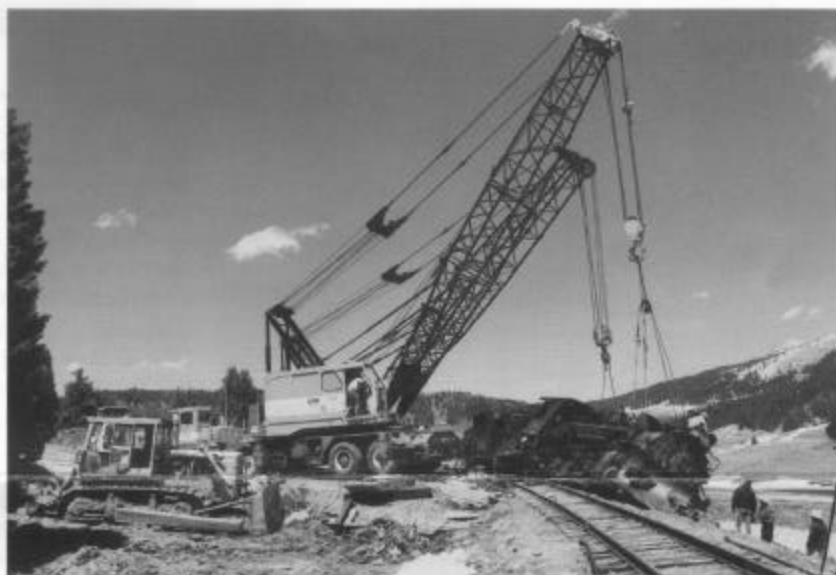
Two, 120-ton cranes in position and ready to lift engine 484 back onto the rails, May 13, 1999. (All photos by Tom Cardin.)
