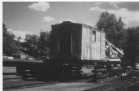
The superstructure on cribbing with the flat car removed, before being lowered onto a flatbed truck for the trip to Colorado Springs. (Ken Spencer)
