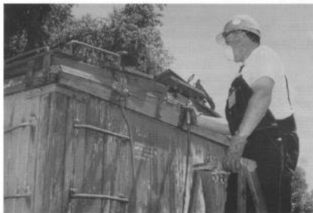
Don Stewart paints 30-foot refrigerator car 55 in Chama (session B). The painting crew scraped and painted eight cars in the two June sessions.
