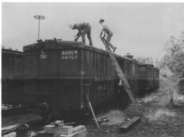
Scott Leidenberger (left) and Lisa Leidenberger work on replacing the roof walk of cable car 04426 in the east Chama yard (session B).
