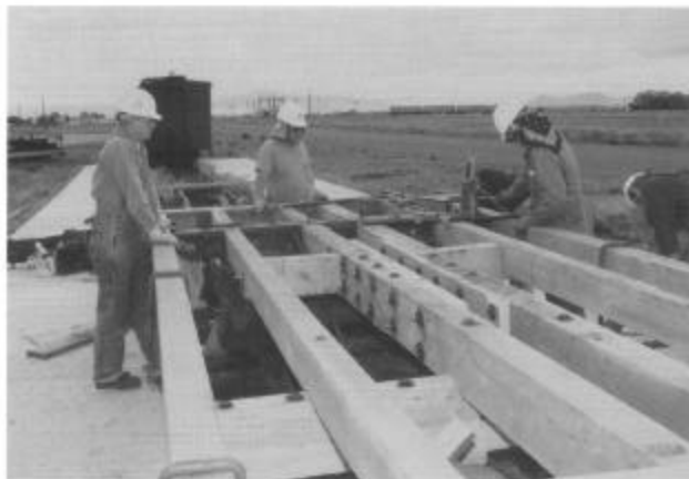
In Antonito during session A, Keith Hayes (left) and Tim Smith watch Bob Hayes use a jack to raise a timber into place so it can be bolted to the frame of flat car 6708. In the foreground, a similar timber has been bolted in place. (All photos by Tom Cardin except where noted.)
