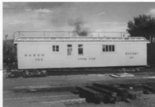
Railway Post Office (RPO)/Cook Car 053 in the Chama yard at the end of the June work sessions. Volunteers completed the end platform work begun in 1997 by installing new steps. They also relettered the car. 053 was built as a 30-foot RPO in 1885 and served for many years on the Chili line between Santa Fe, New Mexico, and Alamosa, Colorado.
