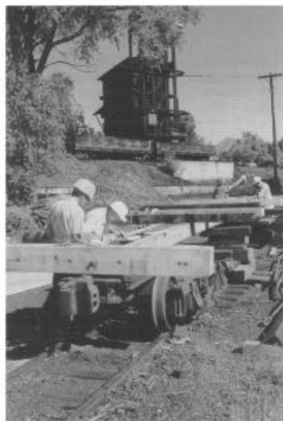
Don Bush (left) and Geof Gordon work on the center sills of flat car 6214 in the east Chama yard. In the background are Jim Phelps (left) and Fred Springer (session C).
