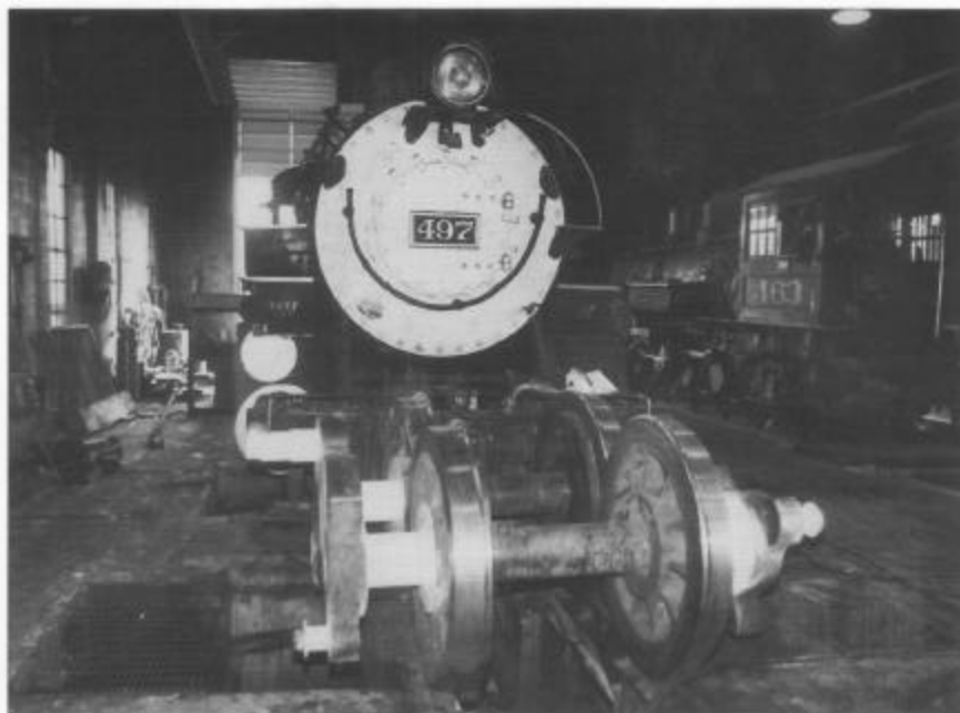
Thanks to the efforts of Friends Phil McDonald, Jerry Sahnd, Gerald Blea, Roger Briggs, and Mark Yates, freshly painted locomotive 497 sits in the Chama enginehouse awaiting the installation of the drivers—two sets are in the foreground. The team spray painted the locomotive in the Chama enginehouse on February 26, 2000. (Photo by Tom Cardin.)
