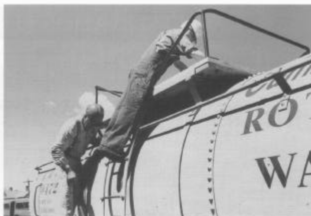
Chuck Templin and Bob Craine working on the new wood decking of Rotary Snowplow OY's water car.
