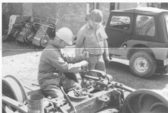
With the trucks removed from the short refrigerator car, Jay Samuels (left) and Randy Worwag work on the brake rigging (session C). (Tom Cardin)
