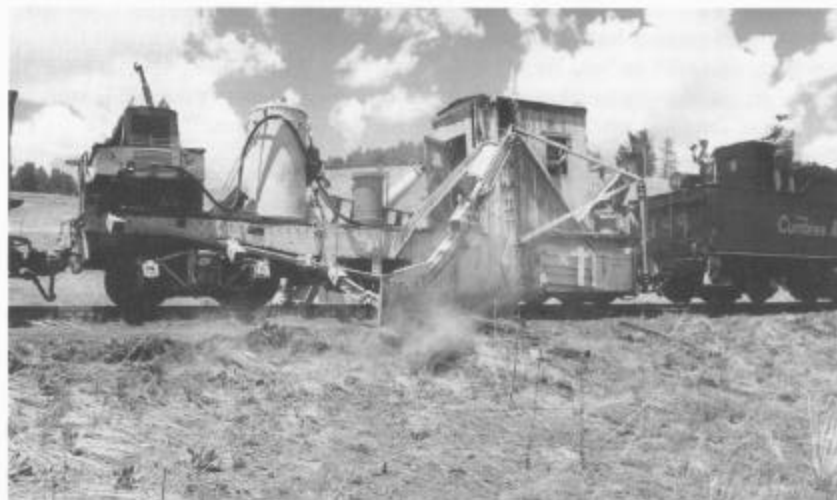
The Jordan spreader clears a wide swath along the track on June 5, 2000, as part of the railroad's extensive fire prevention measures this past year. The work extra also included engine 487 and caboose 05635. (Photo by Tom Cardin)
