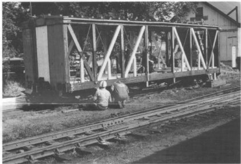
In the Chama yard, coach 209 being converted back to its configuration as boxcar 3605. The car was built in 1904 and rebuilt at Alamosa in 1924-1925. The car ends have been sealed and the bracing replaced. Volunteers also installed a new floor (session A). (All photos by Tom Cardin except where noted.)
