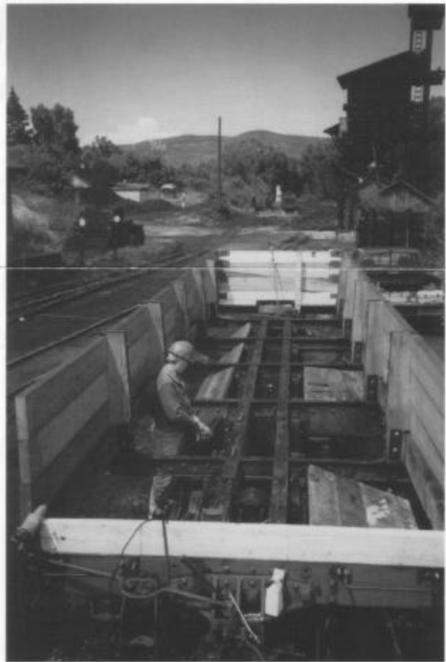
Looking north in the Chama yard, work session C, August 8, 2001. The restoration of drop bottom gondola 727 is almost complete. (Photo by George Swain.)
