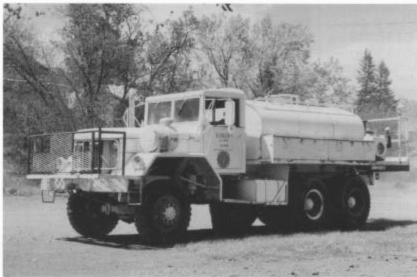
The new fire truck for the C&TS, before its coat of red paint. Four and one-half-ton, with six-wheel drive, the truck can "go anywhere" to put out fires (May 2002). (Photo by Tom Cardin.)
