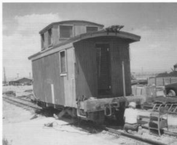
Short caboose 0579 in the Antonito yard during session C. The crew is installing the coupler on the B end of the car (the coupler pocket has been attached to a new oak end beam). Note the new wood siding.
