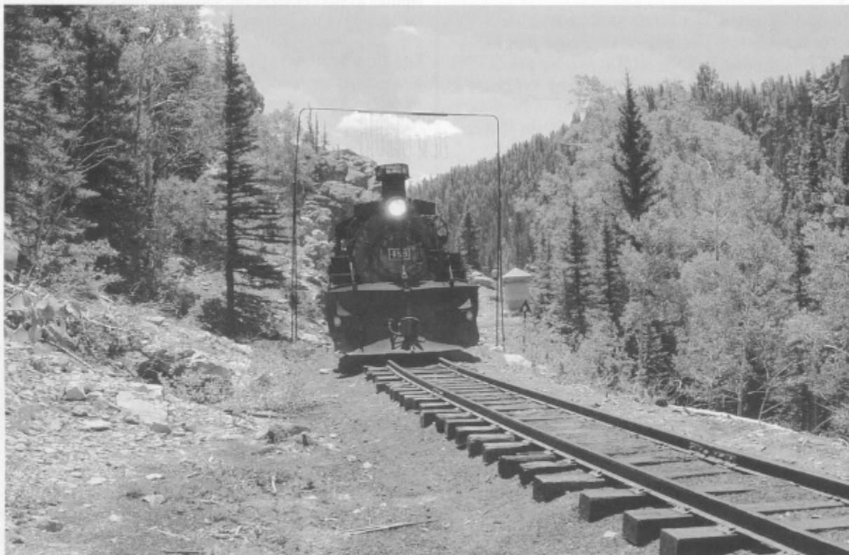
*The first train to run under the newly installed tel'tales at Rock Tunnel. (Team photograph)*
