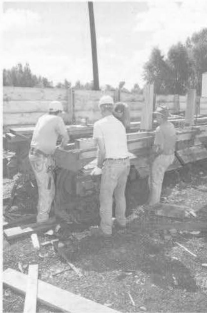
Roy Blizzard, Tony Kassin, Dale Johnson, and Tim Bristow fit last door to the drop bottom gondola. (Tom Cardin)
