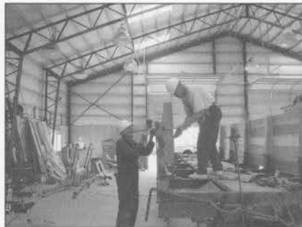
Warren Ringer and Bill McCartin clamping a side board to a side stake before drilling holes for the bolts.
