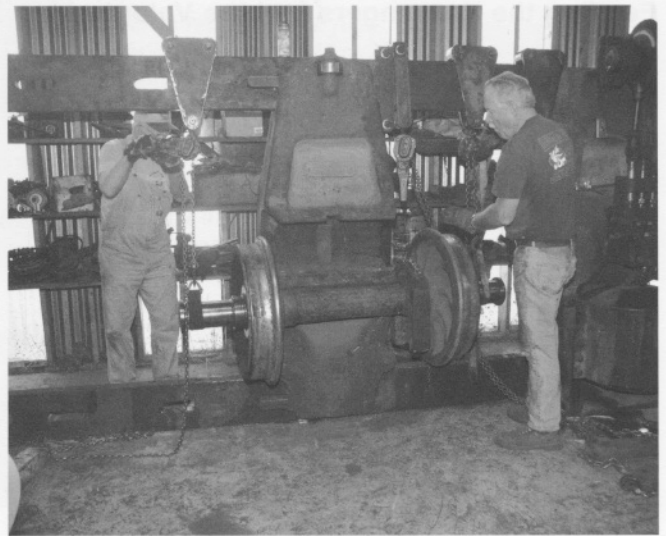
Les Clark and Jim McGee lifting wheels into the wheel press to remove the cast iron wheels from the axle. (Tom Cardin)
