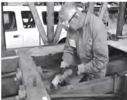
Terry Boardman grinds flash from the steel brackets that attach the caboose structure to the new steel center sills.
