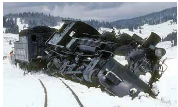
While clearing snow and ice on April 25, 1999, C&TS 484 (lettered for D&RGW photo charters) hit ice in the flangeway and derailed just west of the Los Pinos tank. Fortunately no one was injured but the engine was close to rolling over. Due to damage, it did not see service again until 2004. Photo by John B. West, FCTS, JW02-012
