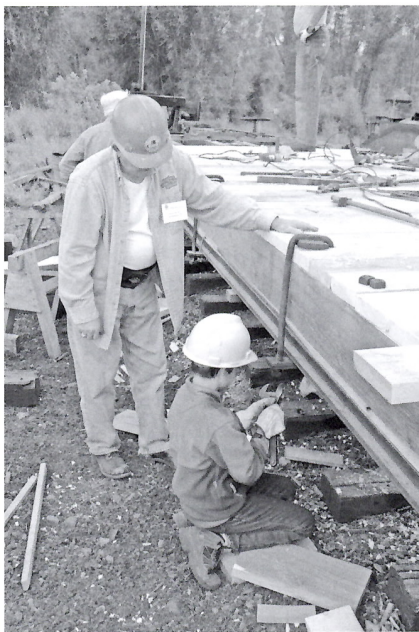
Dave Sands watches as his grandson, D.J. Sands, tightens a U- bolt on the idler car.
