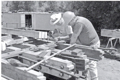
Dan Robbins and John Ruhr working on sill of car 3553.
