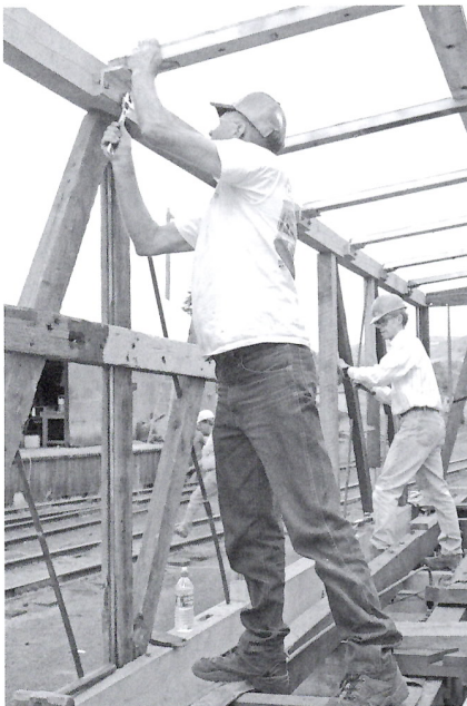
Bob Lenicheck and Wendell Schweitzer setting roof ribs on car 3553.
