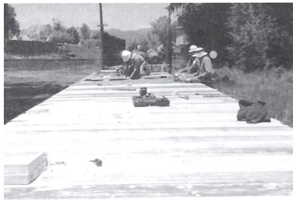
The team members have almost finished installing the new deck boards on flat car 6314.
