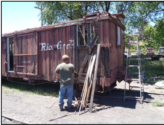
Joe Kanocz removing old siding.
