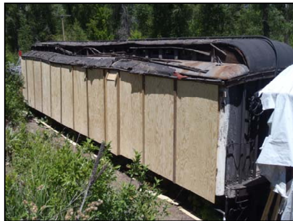
Plywood siding completed on #065.
