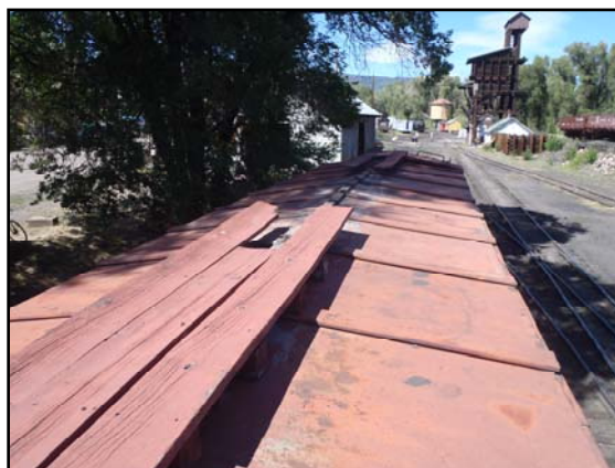
Murphy roof panels have been re-installed.
