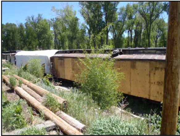
Plywood siding completed on #0452
