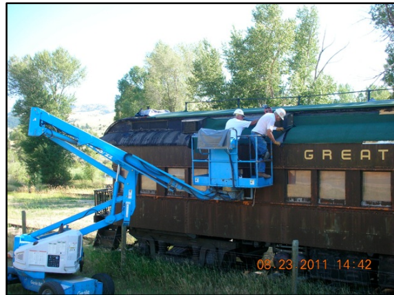
Chuck Deuker and Tarry Rahne putting rolled roofing on A-3
