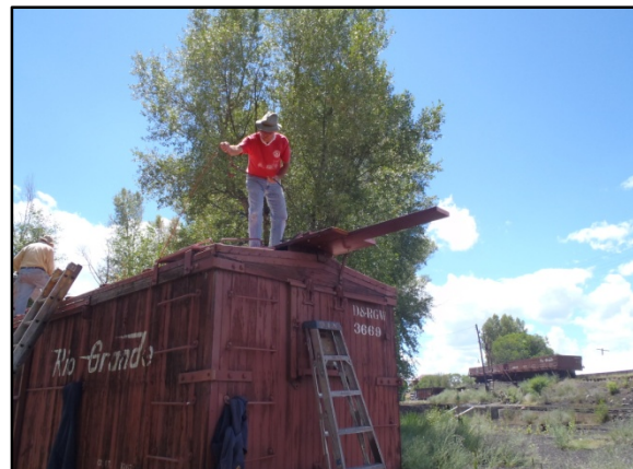
Team Leader Tim Bristow prepares to cut off roof walk boards.
