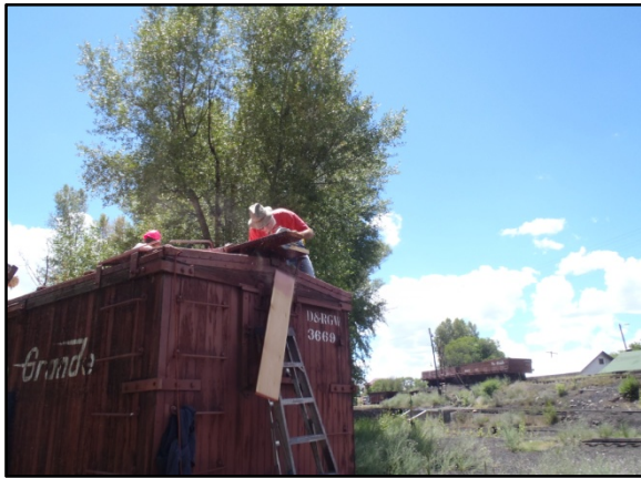
Excess roof walk being cut off by Team Leader Tim Bristow.
