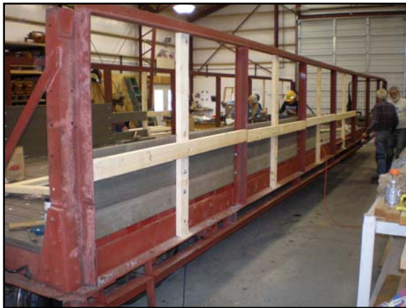
Nailers have been installed.
