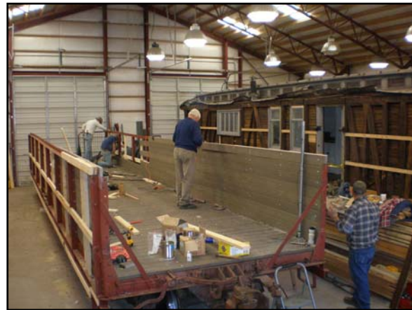
Inside planking well underway.
