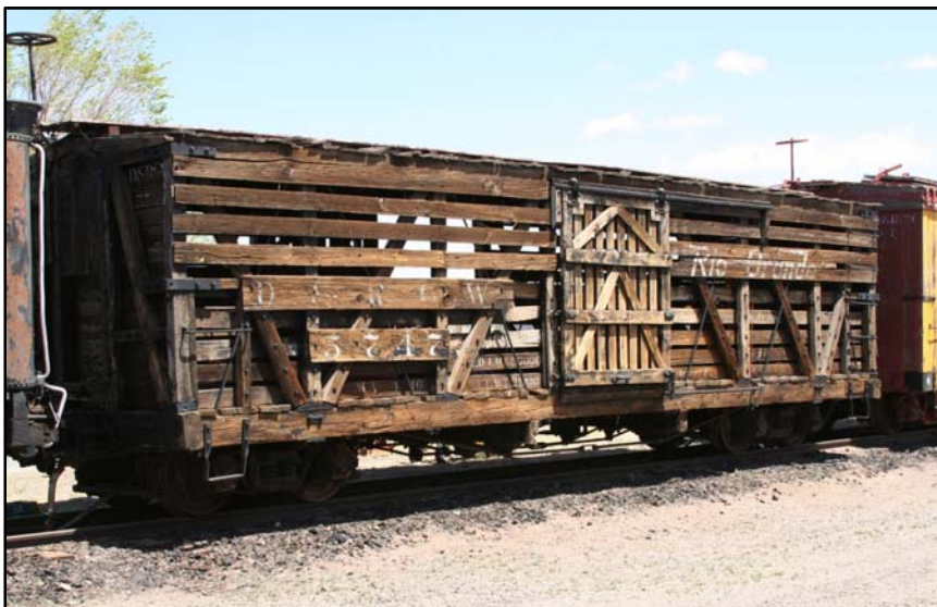
Stock car #5747 was prepared during the A Session. A light scraping was all that was necessary for the primer application.
