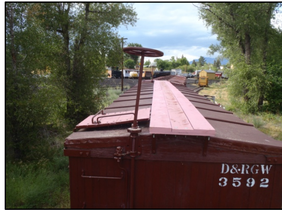
New primed roof walk on car #3592 Still needs a final coat of paint.
