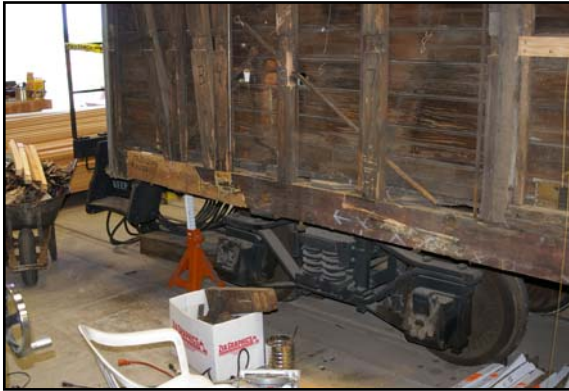
Layout of sill replacement.
