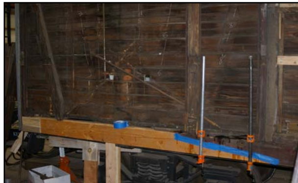
New sill section in, end sill repaired, epoxy
