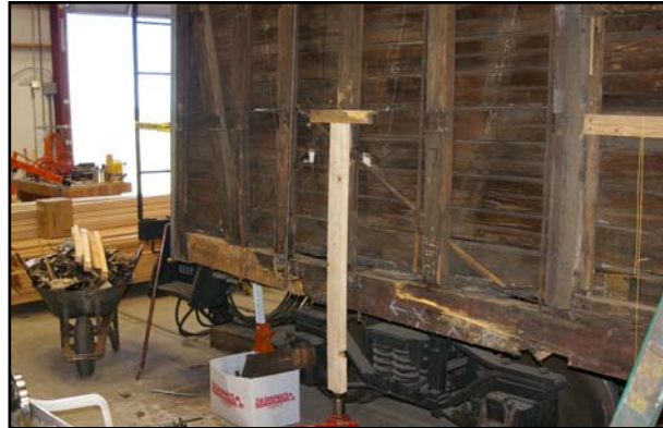
Jacking up side of car to release tenons.
