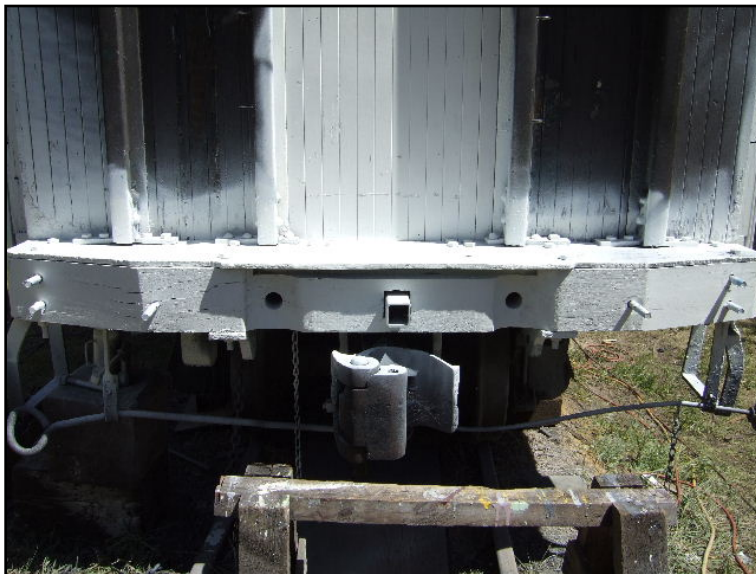
End sill B end installed.
