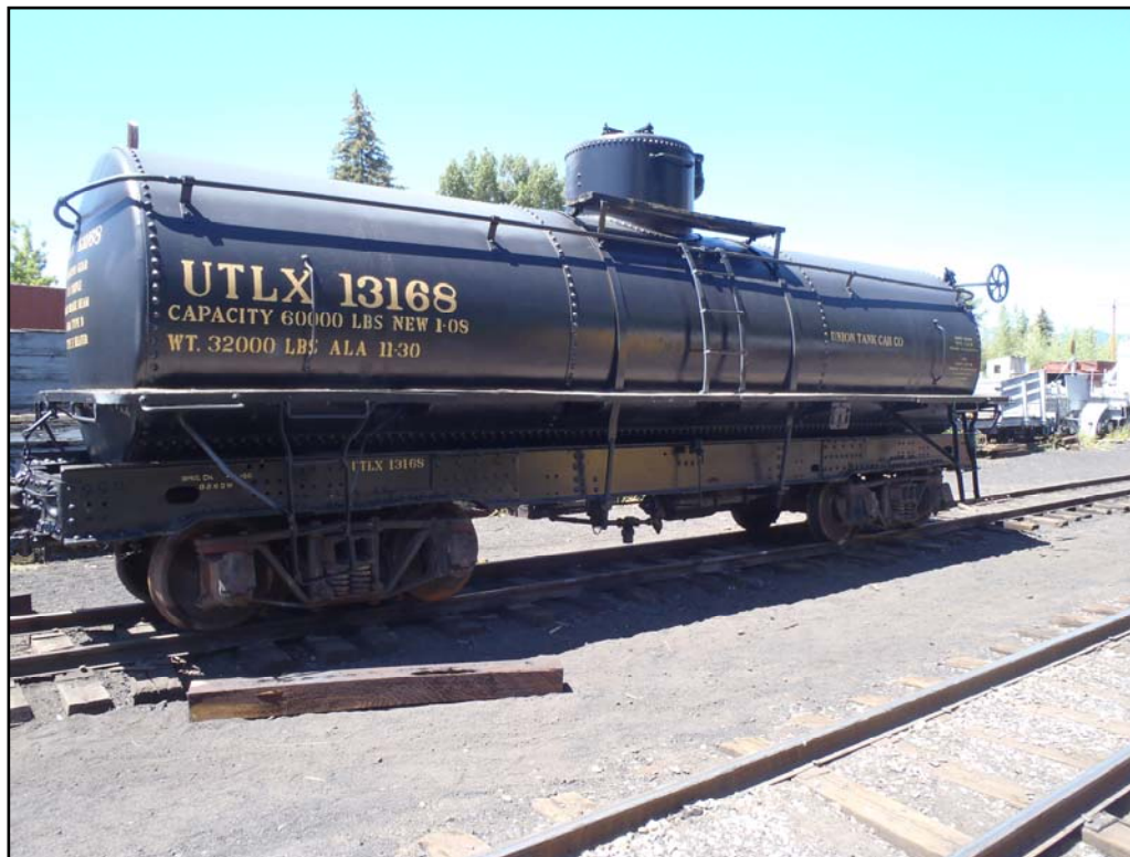
Archbar trucks have replaced the Bettendorf trucks on UTLX 13168
