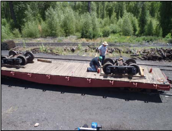
Bettendorf trucks being secured to flat car #6544
