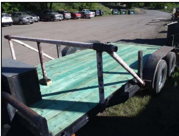
Repaired tool box and new floor was installed. Green.
