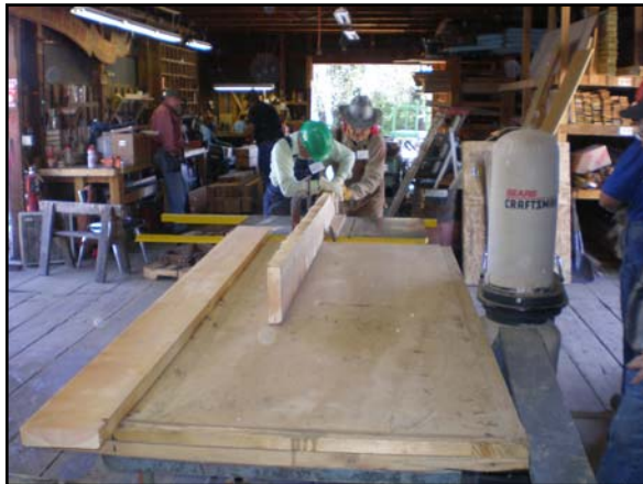
Making cut to make shiplap boards.
