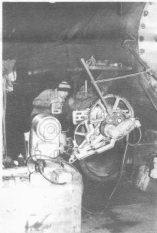
ABOVE: Felipe Samora monitors the valve and cylinder boring bar grinding locomotive No. 487's right-hand valve cage 2\frac{1}{1000} in. per cycle. This reboring of the cages and cylinders has probably not been done for about 30 years. A wheezing rather than a sharp exhaust sound indicates leaking valves.
