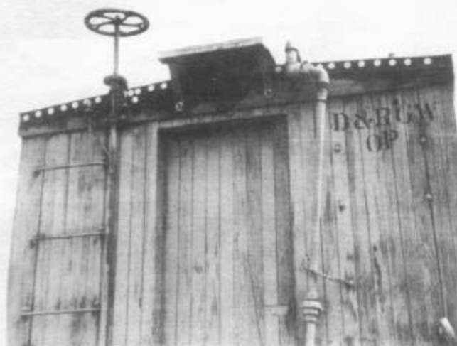
ABOVE: End view of derrick OP showing new braces for roof walk, steam pipe, and reinstalled brake wheel and staff with ratchet and pawl. The edges of the new roof are tacked to the fascia board with nails and roofing washers. The roofing crew for the derrick was Howard Bunte, team leader; Dennis Chiles; Jack Schuh; and Craig Story. The crew also began work on historic caboose No. 0503, built in 1886. Old roofing material on the cupola was removed, a few boards were replaced, and new canvas and tar compound (Indukril) were applied. Photograph by Arthur Nichols.
