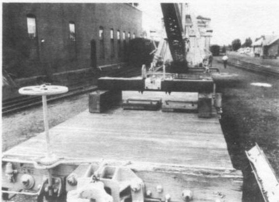
LEFT: Boom tender car with new planking and boom cradle in the Chama yard. The roundhouse and machine shop are to the left. To the right and in the distance is the Chama depot, built in 1899. Photograph by Arthur Nichols.
