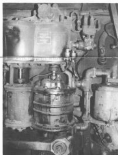
The air pump on 487. The air compressor governor is to the upper right, with the steam pipe disconnected. February 11, 1997
