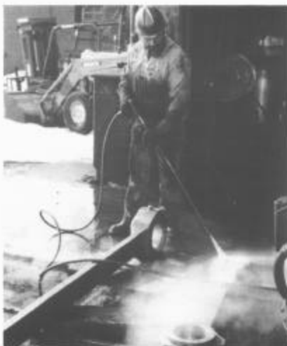
In the Chama engine house, Tommy Garcia uses a high-pressure cleaner on rods in preparation for bearing inspection. February 11, 1997
