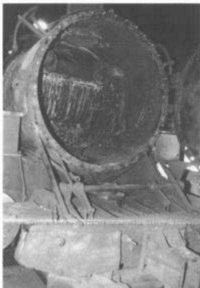
Say ah! 487 with smokebox open for flue check. Note the superheater elements. January 17, 1997
