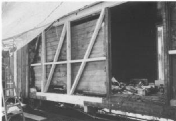
Refrigerator car 157 with new sections of header and outside main sill and new uprights and diagonal braces. Al Smucker photo.
