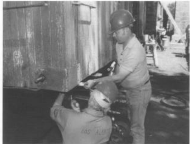
In Chama, Jay Samuels and Randy Worwag attach a plumb string to refrigerator car 55 in preparation for tightening the truss rods. The crew worked long and hard through Saturday morning to finish.
