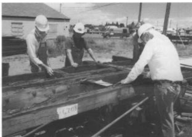
Warren Ringer (left), Bill Kepner, and Wayne Freeark look over rotten wood on flat car 6708 in the Antonito yard, August 1997. Tom Cardin photo.
