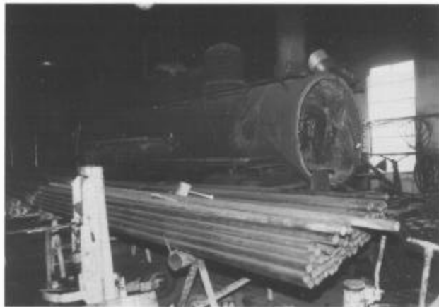
Flue tubes for the 487 on the rack in front of the 463 in the Chama enginehouse, December 1998.
