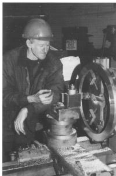
Bill Jeffcoat turns a bronze piston ring in the Chama enginehouse, January 1999.
