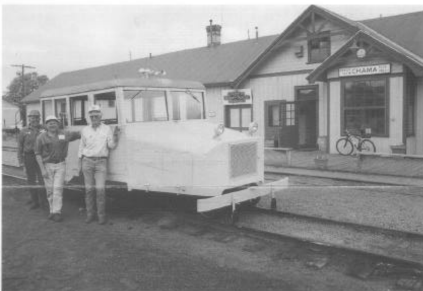
Restoration of inspection car MW02 was completed during the June work sessions. Here, Gus Wurtzer (left), Don Huber, and Joe Phelps stand beside MW02 parked in front of the Chama depot on June 30, 2000. Originally built by Fairmont, probably in the 1930s, it is powered by a Ford V-8 of about 1947 vintage. Restoration began in 1996. (All photos by Tom Cardin except where noted.)
