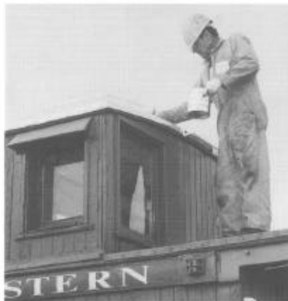
Jack Salisbury applies aluminum water-proof paint to the cupola of caboose 0503, an original D&RGW caboose (session A).
