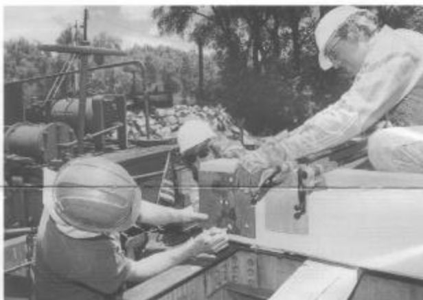
Jeff Smith marks where a hole will be drilled to hold the corner brace on flanger OJ, while Sherrie Rider and Terry Rider help hold the corner brace (session A).
