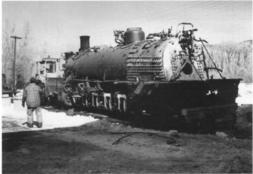
Ricky Rivas guides the loader as it pushes locomotive 484 back into the Chama enginehouse on February 20, 2002. The engine was moved outside earlier in February so that the cab could be removed, allowing access to the staybolts. The narrow-gauge shop trucks help support the locomotive; only the lead and trailing trucks are on the rails. The drive wheels have been removed. (Photo by Tom Cardin.)
