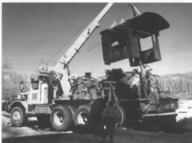
Removing the cab from 484 requires a bit of extra equipment. Steven Butler guides the cab to clear the boiler and valves. The cab must come off to get to the staybolts. Originally there were doors on both sides, but they were riveted and welded shut many years ago (February 2002).
