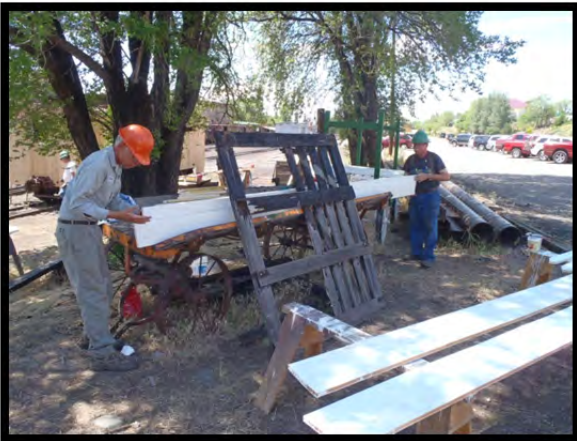
George Detwiler and Scott Stover (sheep stock car #5633) priming roof walks.
