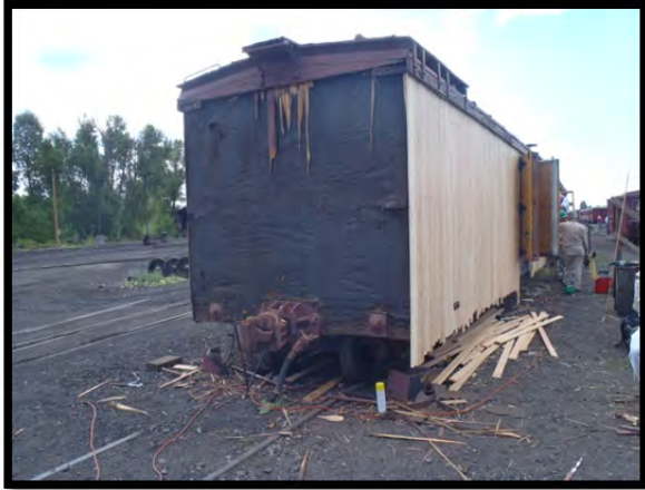
Old siding has been removed from the end.
