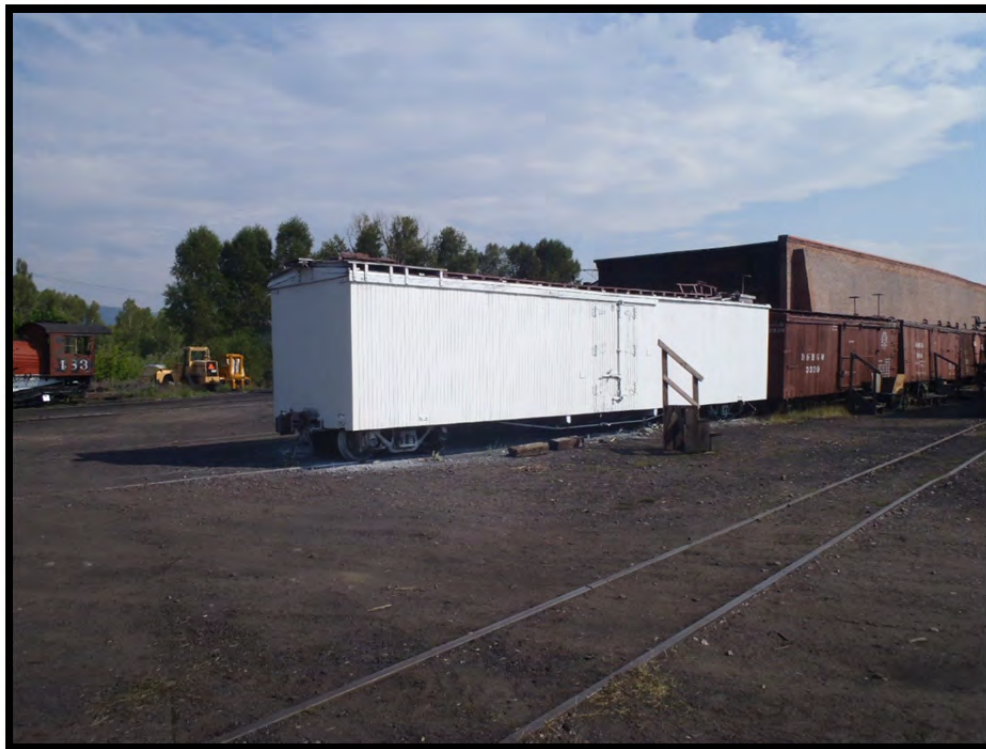
Old siding has been removed from the end.
