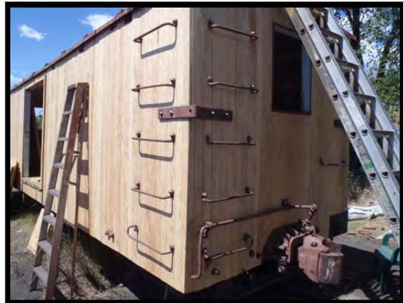
Car has new t&g siding installed along with most hardware like the grab irons, middle braces, etc.
