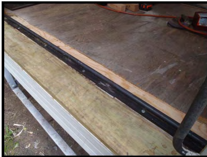
One floor door rail installed in the RPO Car.
