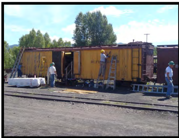
Old siding being remove as well as fascia.
