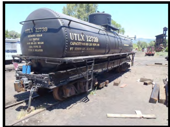
Archbar trucks installed on both ends. 65
