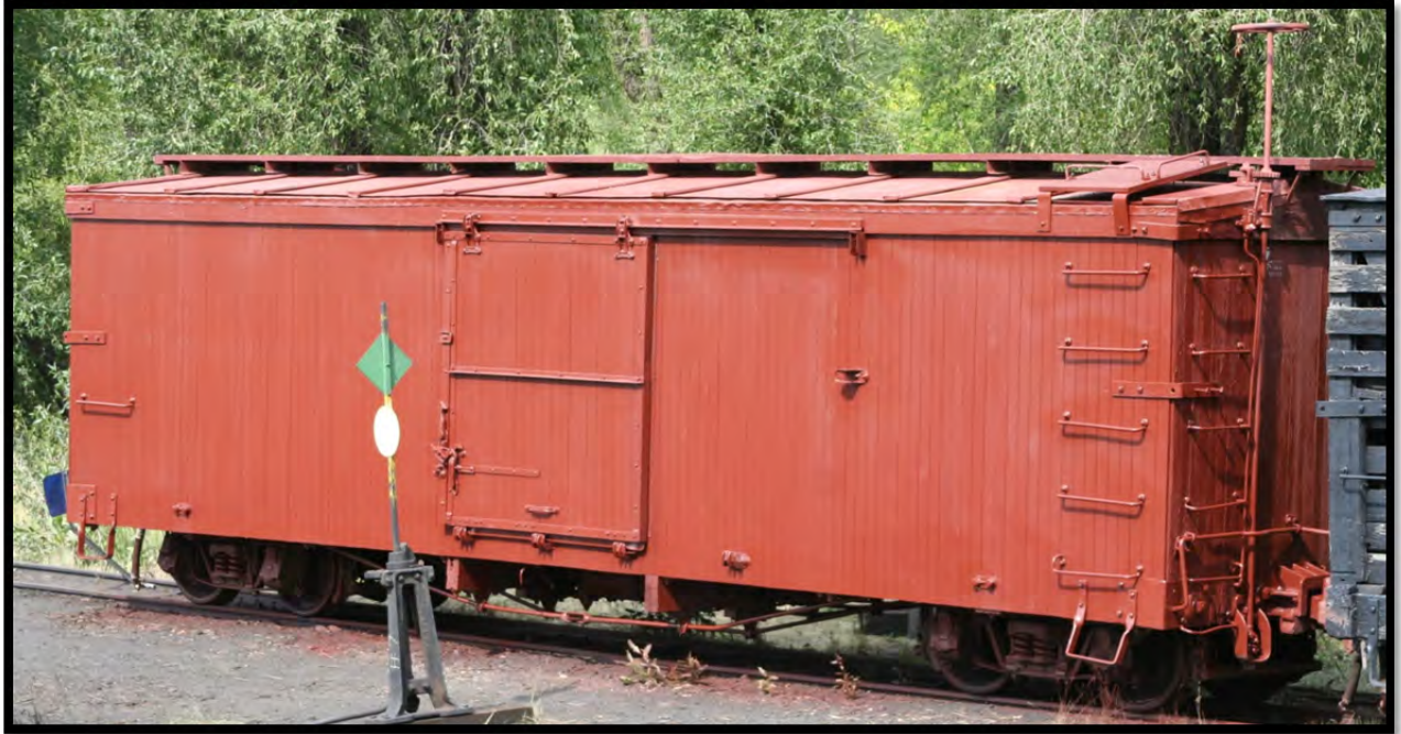
Boxcar 3669 after a finish coat was applied to the sides and ends.
