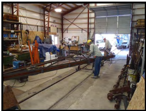
Team laying out angle iron cross bracing to be welded.
