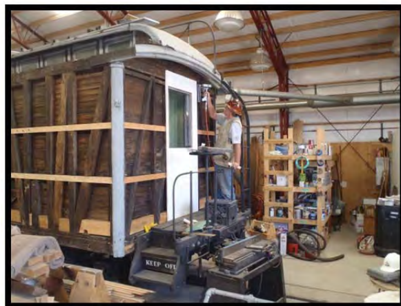
TL Craig McMullen air nailing new white painted siding.
