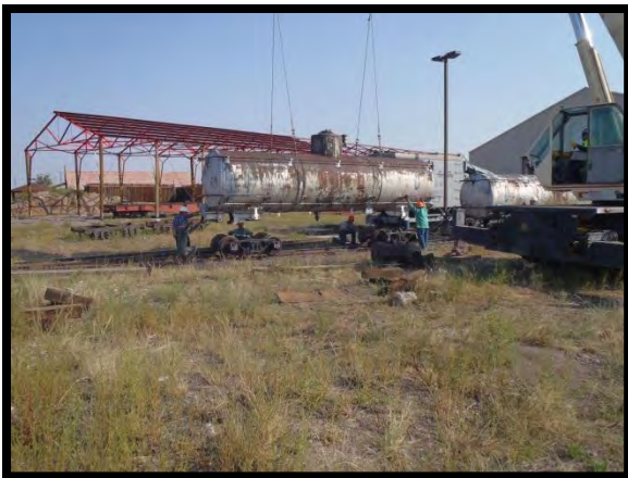
Crane lowering the tank onto the trucks.
