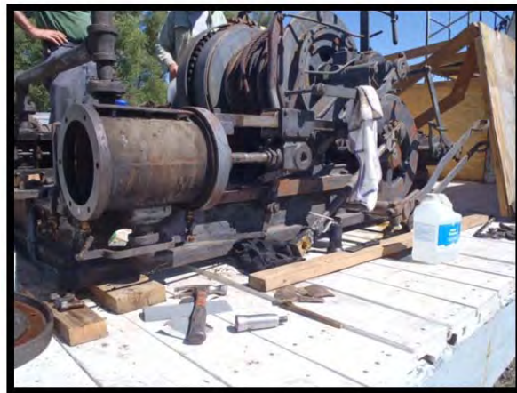
Side view of the two cylinder steam engine.
