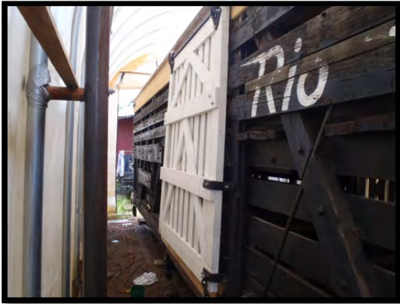
Built new doors for both sides of the car and replaced door tracks and door stops.
