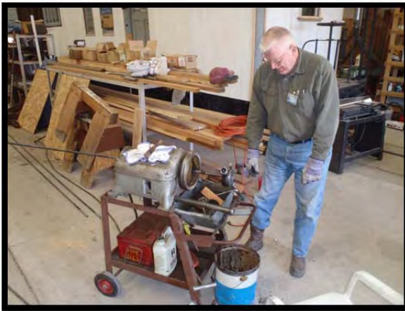
Marshall Smith putting threads on a rod that will be used as cross bracing.
