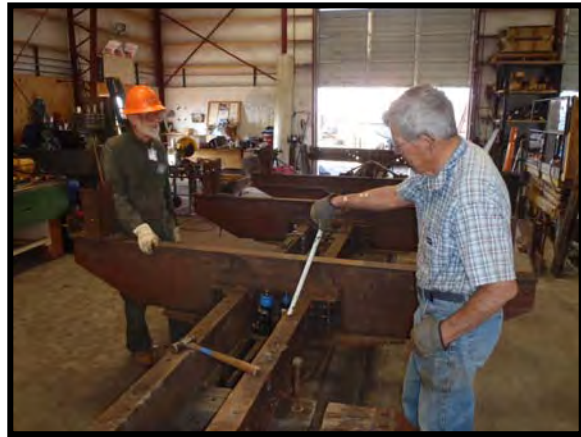
Warren Ringer watches as TL Bill Pratt is preparing to separate a cross-frame from the main frame utilizing hydraulic jacks.
