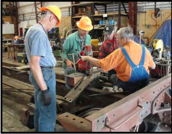
Removing a bolster saddle. (Photo by Bill Pratt)
