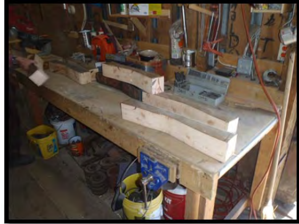
New roof walk supports cut out of one piece of lumber.
