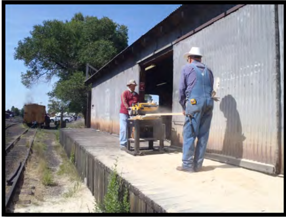
George Davies and L.D. Osborn plane a board to the right thickness for a door.
