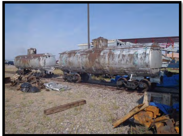
Both frameless tank cars back on trucks for first time in many years.
