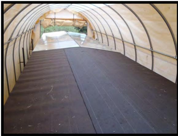
Felt paper was put on top of the new wood roof before the metal roof was put on. This should make the roofs of stock cars last a whole lot longer.
